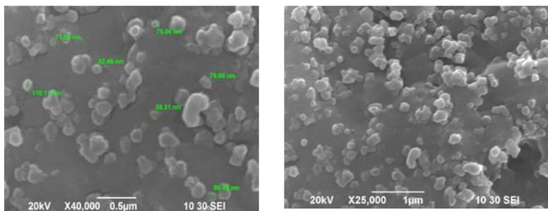
**Figure 2.** SEM images of synthesized titania with different magnification
