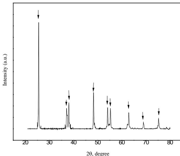
**Figure 1.** XRD spectra of synthesized titania
