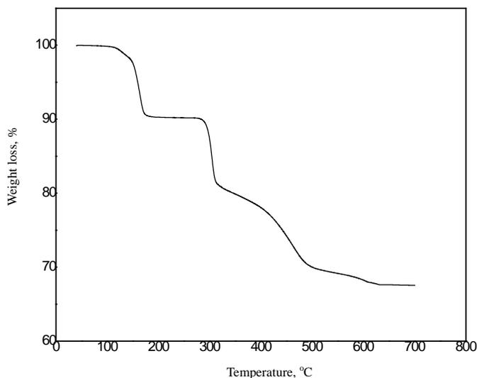
**Figure 6.** Thermogram of synthesized titania
