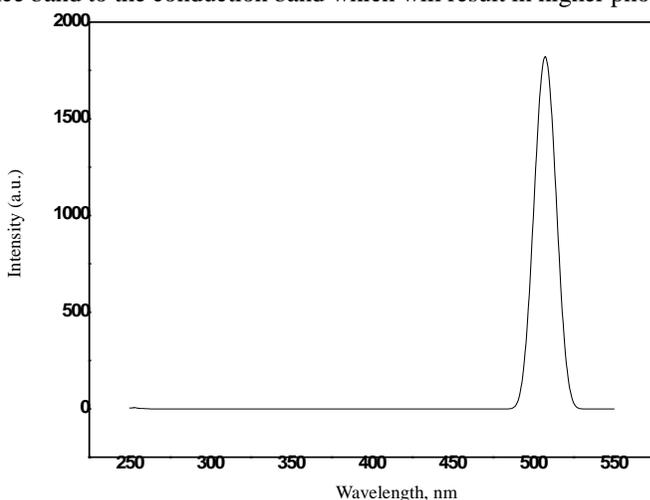
**Figure 5.** Fluorescence spectra of synthesized titania
