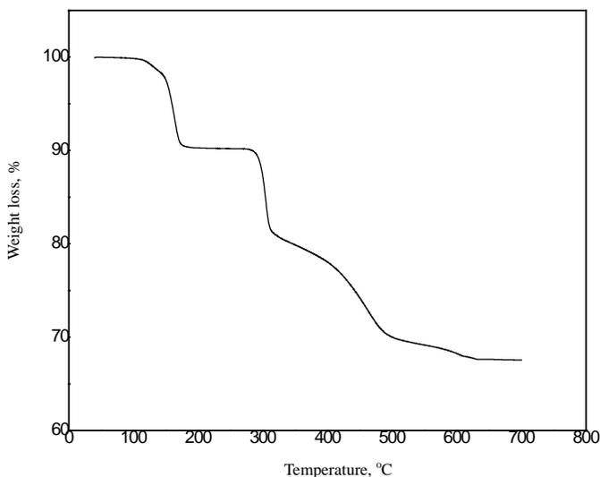
**Figure 6.** Thermogram of synthesized titania
