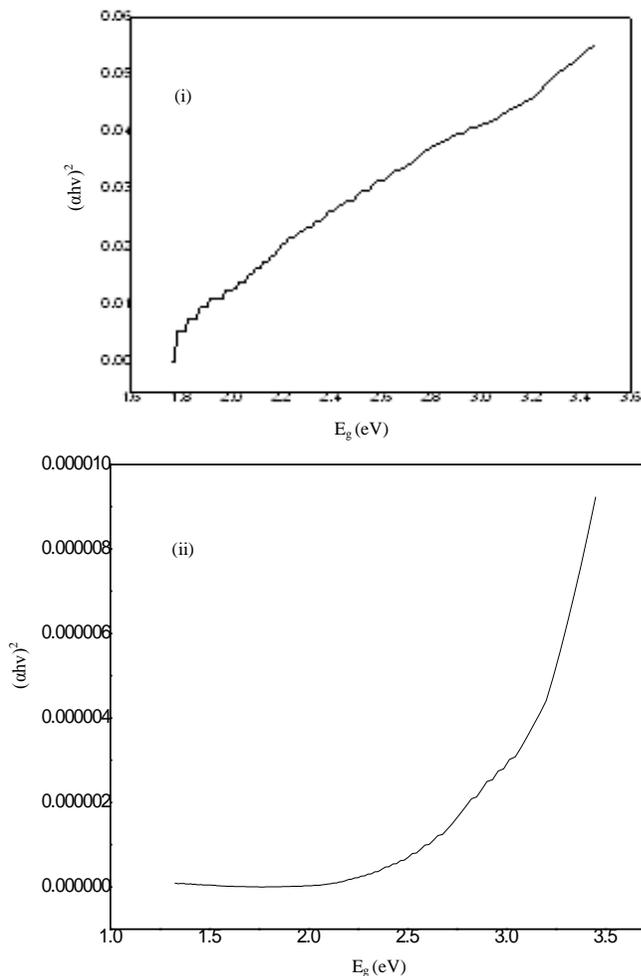
**Figure 4.** (i) UV-Vis spectra and (ii) Band gap plot of synthesized titania
