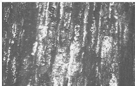
Figure 4 (a): -Mild steel sample blank kept in 1 M HCl for 24 hours at 35 0 C.
